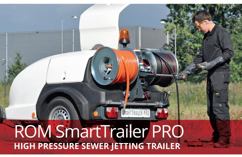
It's here: The new SmartTrailer PRO sewer jetting trailer. Packed with smart solutions based on over 35 years of experience the Smart Trailer Pro is perfect for unblocking and cleaning of sewer lateral lines and main lines up to Ø400mm. Options include petrol or a diesel engine, a cleaning pressure of up to max. 200 bar and a water capacity of up to max. 60 l/min.
