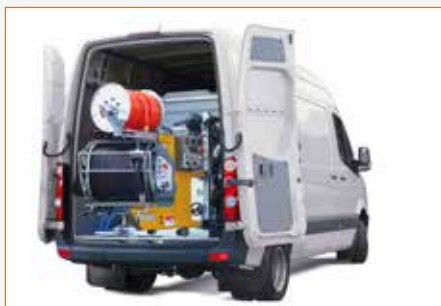
ROM Ecofit HP Skid mounted jetting unit
